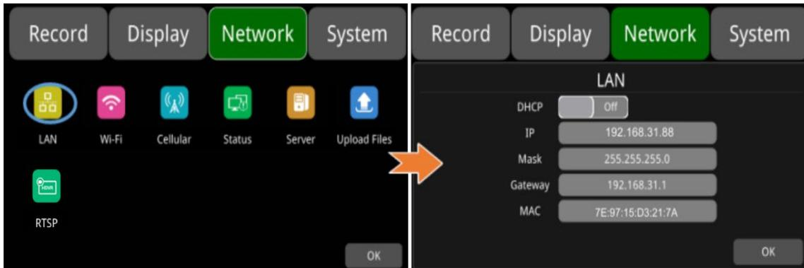
Step 3: If DHCP is set to ON, a dynamic IP will be automatically matched. If DHCP is set to Off, input the IP, mask, gateway and MAC manually.
